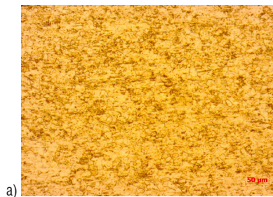
Fig. 6. Investigation of a) the microstructure, and b) chemical compositions of Ti6Al4V; produced by EDX results
