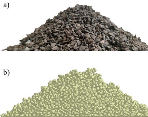
Fig. 10. Comparison of a) actual repose angle, and b) simulated repose angle
