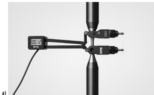
Fig. 2. Setup for creep tension testing with; a) elongation measurement, and b) torsion bar specimen
