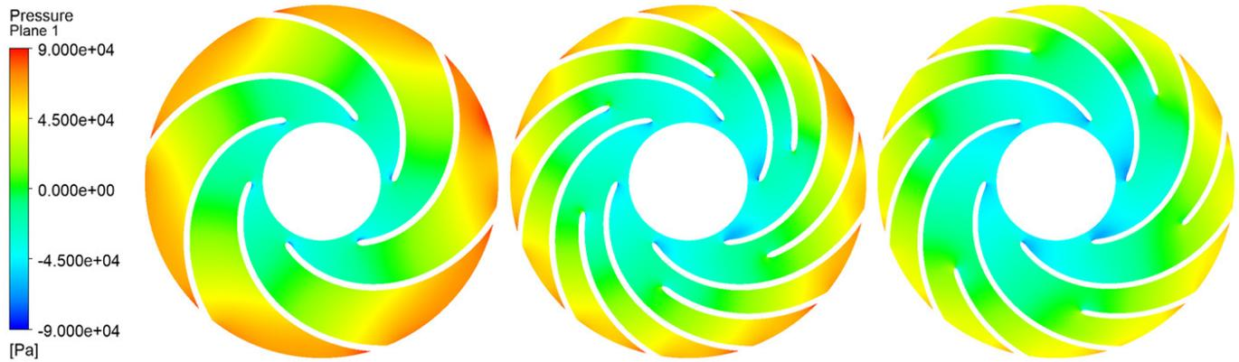
Fig. 9. Pressure distribution in different kinds of impeller
