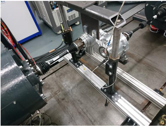
Fig. 4. Gearbox in the test bench
