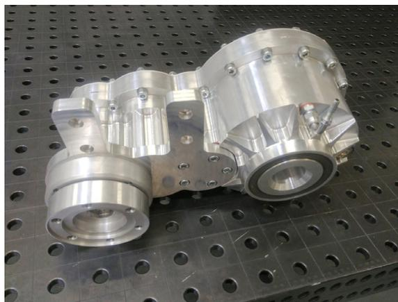
**Fig. 1.** Tested gearbox for the autonomous battery electric modular platform
