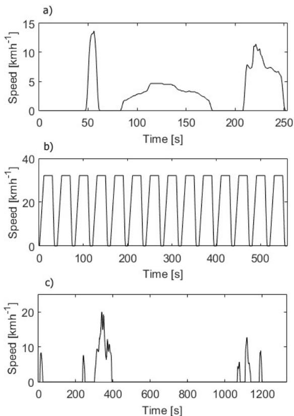
**Fig. 3.** Speed profiles of investigated driving cycles, a) CARB Heavy Heavy-Duty Diesel Truck (HHDDT) Creep Segment, b) Central Business District (CBD) Segment of the Transit Coach Operating Duty Cycle, c) NREL Port Drayage Creep Queue Cycle (California)
