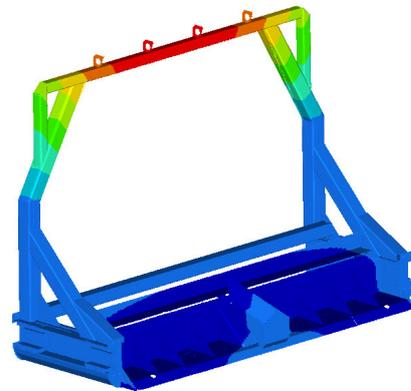
Fig. 8. Static deformation of the ejector plate skeleton
